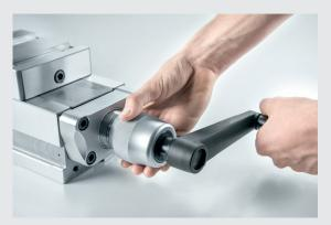
2. Hold the handle tightly and turn the regulator to the desired clamping force presetting step
