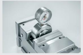
1. Make sure that the moving jaw is not in contact with the workpiece
