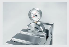
4. Overcome the coupling point and build up high pressure by turning the handle until the stop is reached
