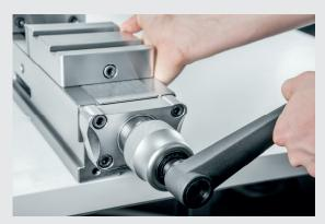
3. Turn the handle until the jaw has contact with the workpiece
